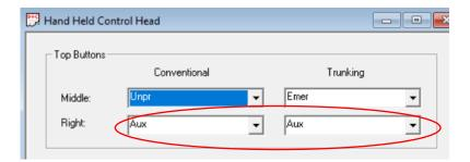
And lastly, you need to enable multi radio system and define if the radio is the primary radio or auxiliary radio, and enter a radio alias for each radio in CPS.
