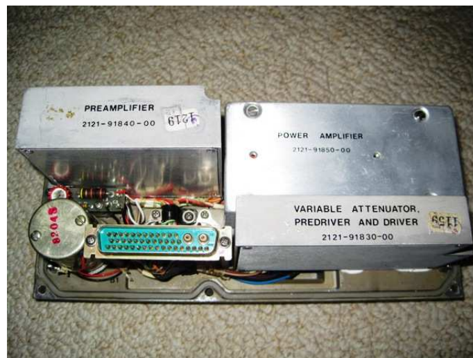
AM-1760 power amplifier assembly
