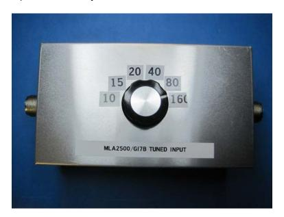
I chose to make my own CM-1 by mounting two six-position selector switches and two SO-239 connectors on an aluminum project box. One switch selects the input side of the filter to be used, and the other switch selects the output side of the filter to be use. The box is connected to the MLA-2500 by as short a piece of coax as practical, and the torroids are "tuned" to that particular length of coax to provide an excellent match.
