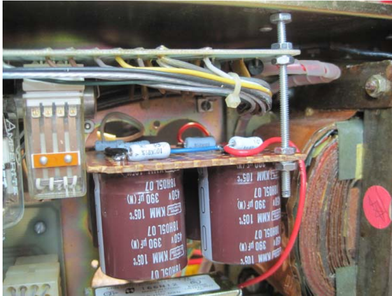
Threaded Rod Holding Filter Board and Control Board To Chassis Bulkhead
